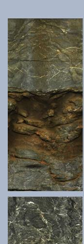
A precision, wide-angle lens and a CMOS camera assembly enable the OPTV52 probe to capture a highdefinition video image of the borehole wall in a variety of horizontal and vertical resolutions.
