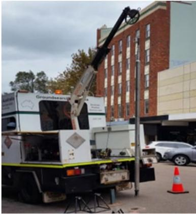
Figure 28 Sonar survey equipment before borehole deployment.
