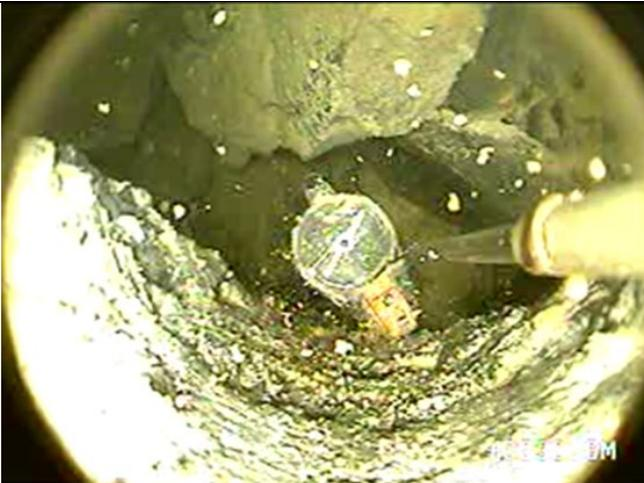
Figure 14 Borehole encountering edge of pillar and room (underwater)
