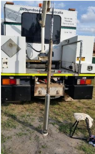
Figure 18 Logging unit setup with laser / video
