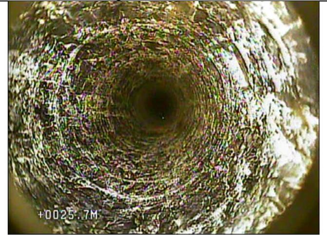
Figure 15 Downward looking underwater view of in place coal in Yard Seam, Newcastle, Aus at 84.3 ft (25.7 m) depth (borehole encountered)
