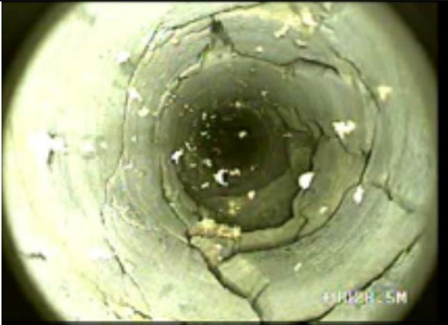
Figure 12 Underwater image of broken rock due to caving (Note suspended particles)
