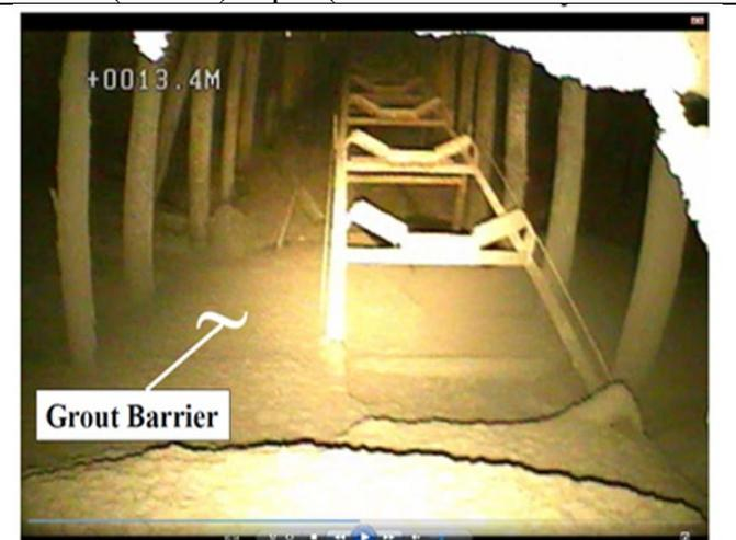
Figure 17 Grout enveloping conveyor in haulageway (Knott et al, 2013)
